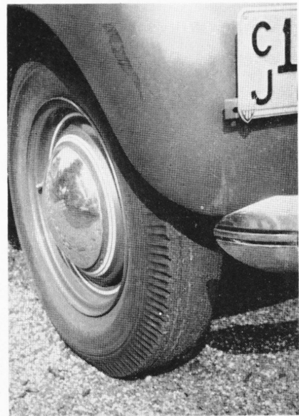
When your tires begin to look like this, it's time to start worrying about them. Recapping is the best answer. There just aren't enough new tires to go around.
